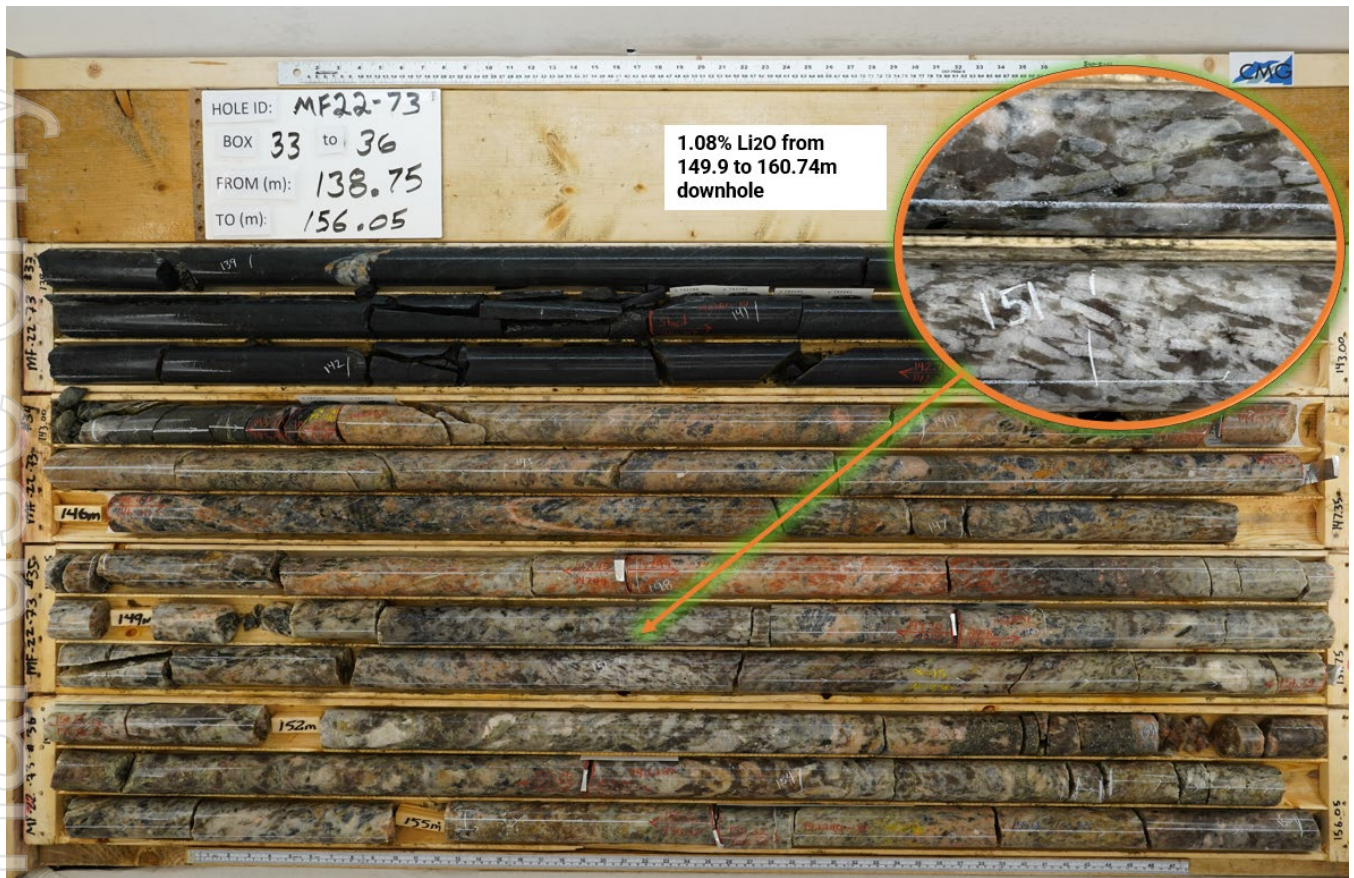
Figure 5: White pegmatite hosts spodumene laths intersected from 143.27 to 160.74m depth in Hole MF22-73.
