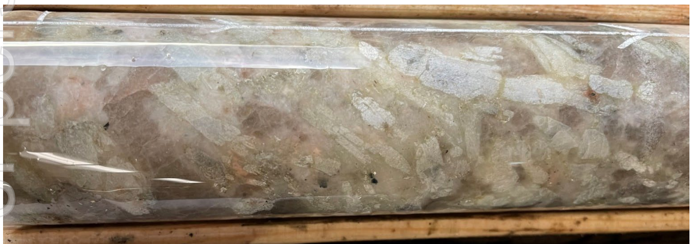
Figure 6: Close up image of white-silver-grey spodumene laths from MF22-80
