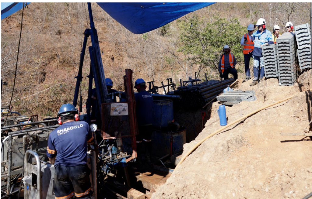
Figure 2: Resource definition diamond drilling rig onsite at the Colina Prospect
