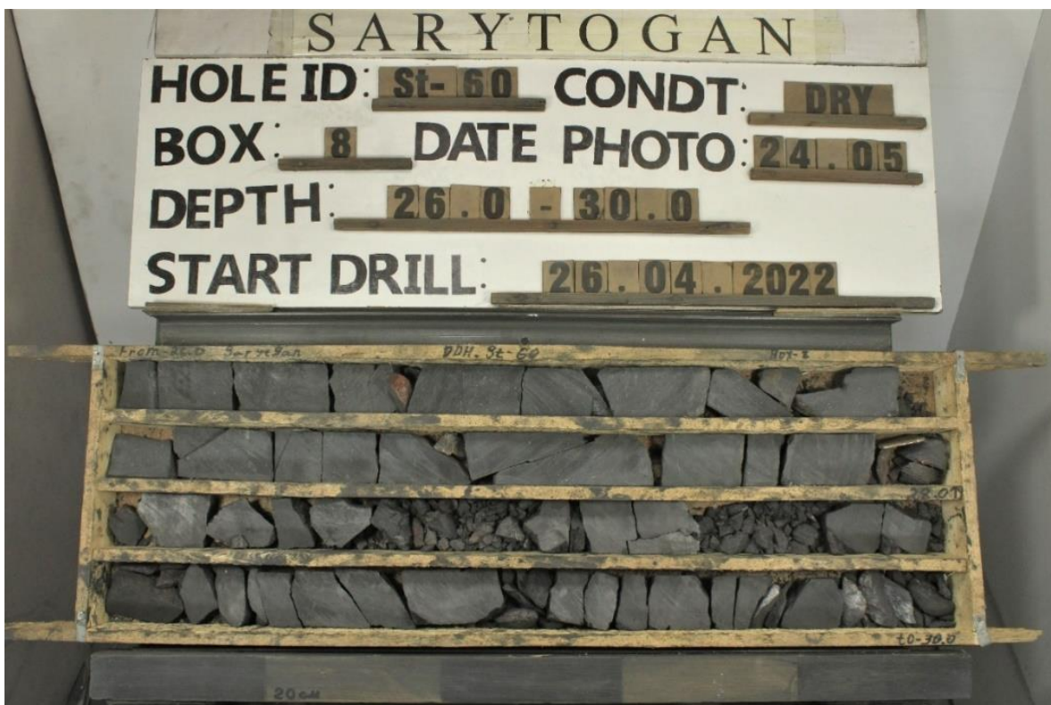
Figure 2 - First High-Grade Graphite Drill Core from the 2022 Program; grading 38% TGC in this interval.
