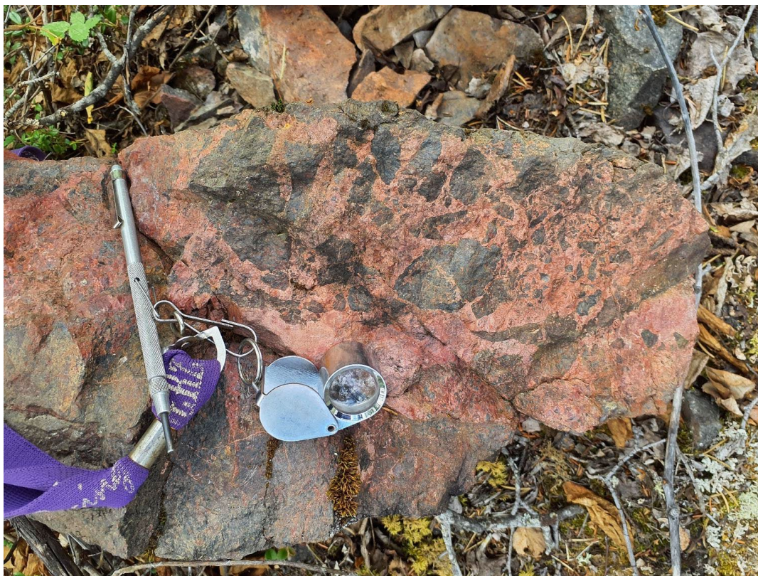
Figure 1: Surprise Creek Fault - Hematitic breccia with U, Cu and Pb mineralisation (max scintillometer reading of 65,535 cps)
