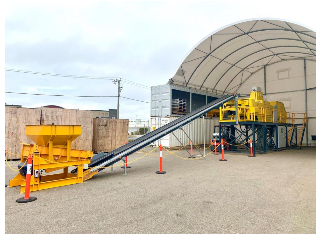
Above: Steinert full-scale ore sorter used for test work in Perth, Western Australia
