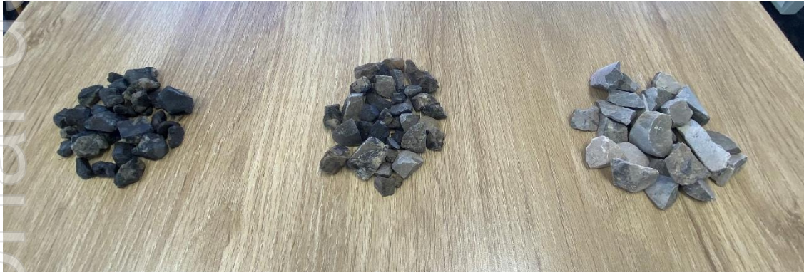
Above: Storm Copper Project – Three ore-sorting products generated from Storm drill core (STOR1601D – 4m @ 4.16% Cu from 97m)
