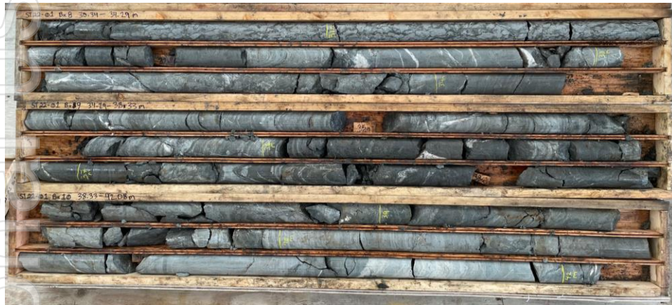
Above: Massive/breccia chalcocite (gunmetal grey) hosted within dolomite (light grey) in drill hole ST22-01 – 2750N Zone
