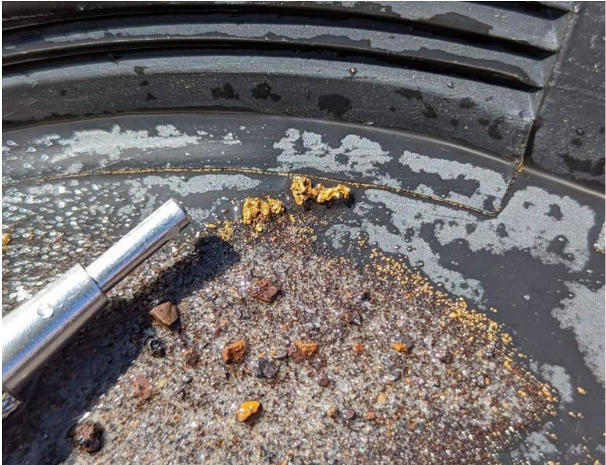
Figure 2: Coarse gold panned from interval 52m-56m in hole 22SAAC061, which returned 4m @ 63.20g/t Au.
