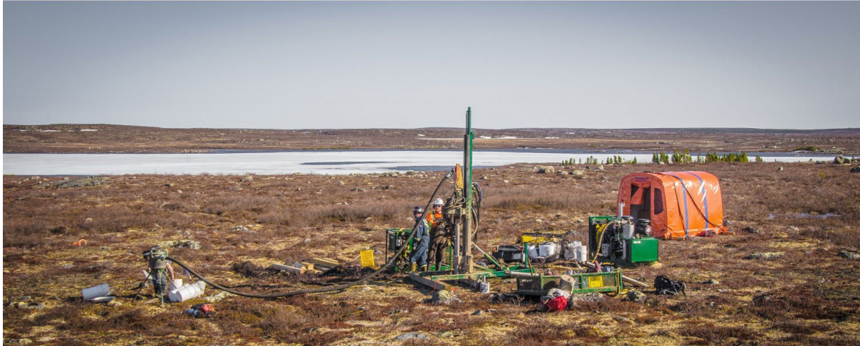
Figure 5 - RC drill rig to be used at Cancet in the autumn drill campaign on a previous job
