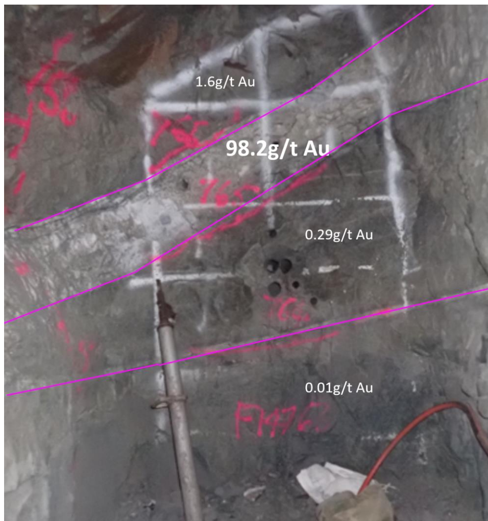
Figure 1: Face photo of the 8 Level McNally Reef from recent underground development
