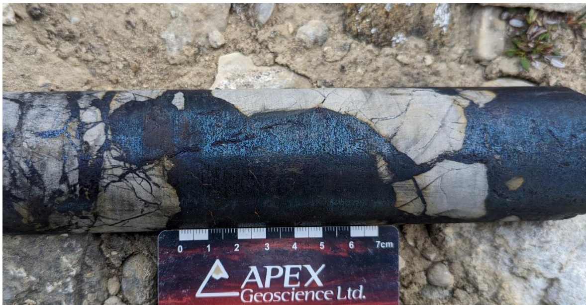
Figure 1: Massive bornite from approximately 50.9m downhole in drill hole ST22-05
