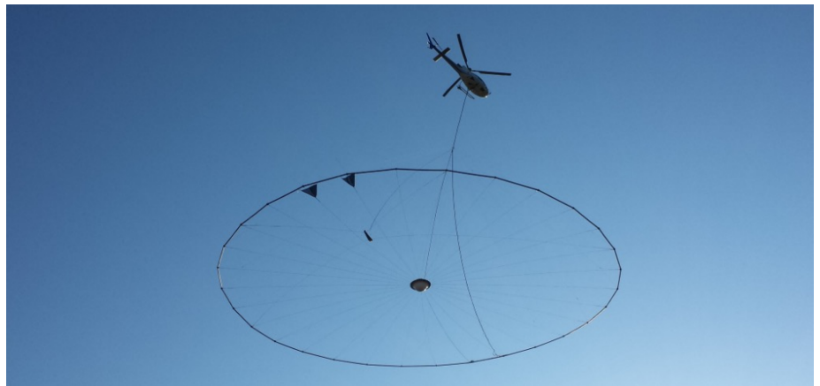
HelITEM 2 helicopter time-domain AEM Survey
