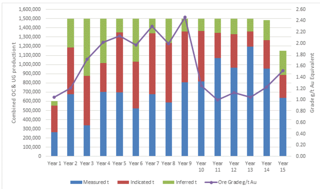
Figure 4: Combined OC/UG Plant Feed tonnes by JORC Category and Grade -1.5 Mtpa
