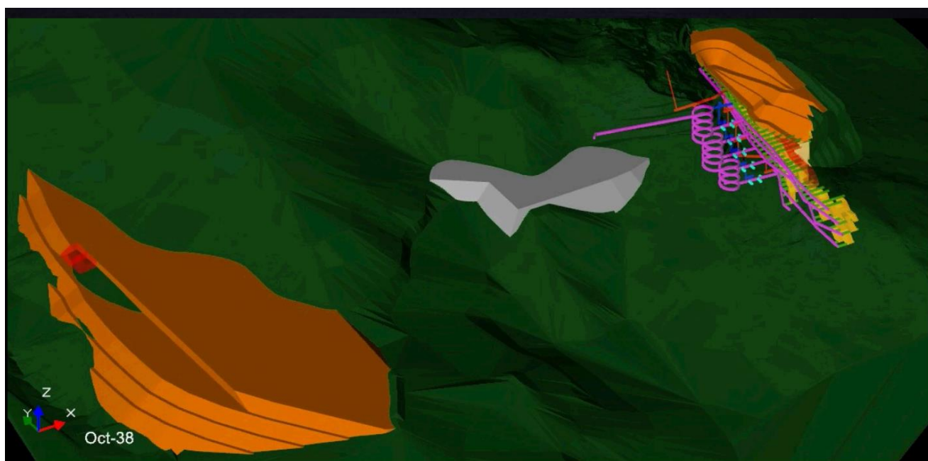
Figure 1: Combined OC/UG Hybrid 1.5 Mtpa throughput – at end of Mine Life (Year 15; Oct '38) – West Waste Dump Prioritised and In-Pit Dumping
