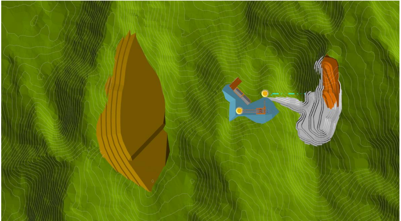
Figure 2: Combined OC/UG Hybrid 1.5 Mtpa throughput – Overall Mine Layout – West Waste Dump Prioritised and In-Pit Dumping
