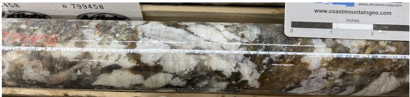
Figure 1: Close up of MF22-116 at 76 to 76.2m downhole. Significant white-grey large spodumene laths
