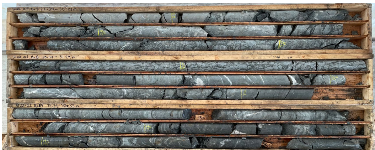
Figure 1: Drill core showing strong chalcocite (copper sulphide) mineralisation between 26.39 and 38.33m downhole in diamond drill hole ST22-01, 2750N Zone, Storm Copper Project
