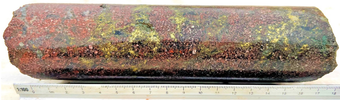
Figure 4 LEFD006 interval 435.6-435.8m showing Burns diorite porphyry altered by pervasive hematite, cross-cut by chalcopyrite and pyrite stringer veining
