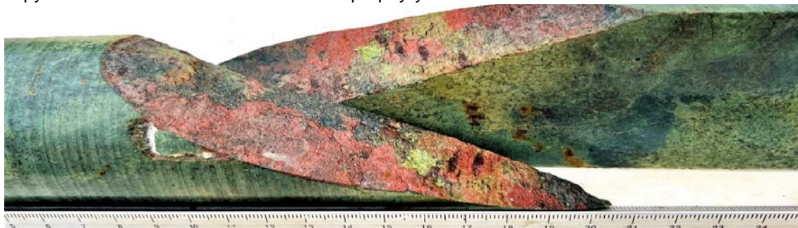
Figure 2 LEFD006 interval 224.5 to 224.8m shows high-magnesium basalt, mineralised by native copper along fracture plane with a gypsum film, with epidote alteration and minor ex-sulphides
