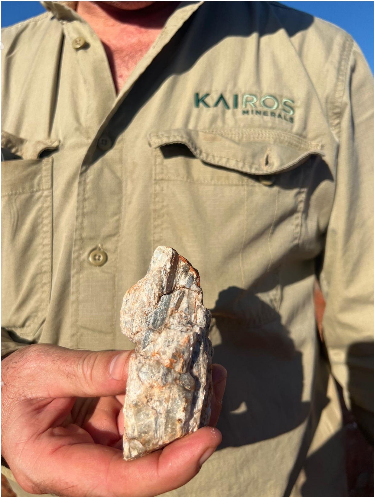
Figure 1. Kairo's Geologist Campbell Watts holding a piece of spodumene-bearing pegmatite (MYR393 - 1.91% Li 2 O) discovered at 'Lucky Sump' during routine earth moving activities.
