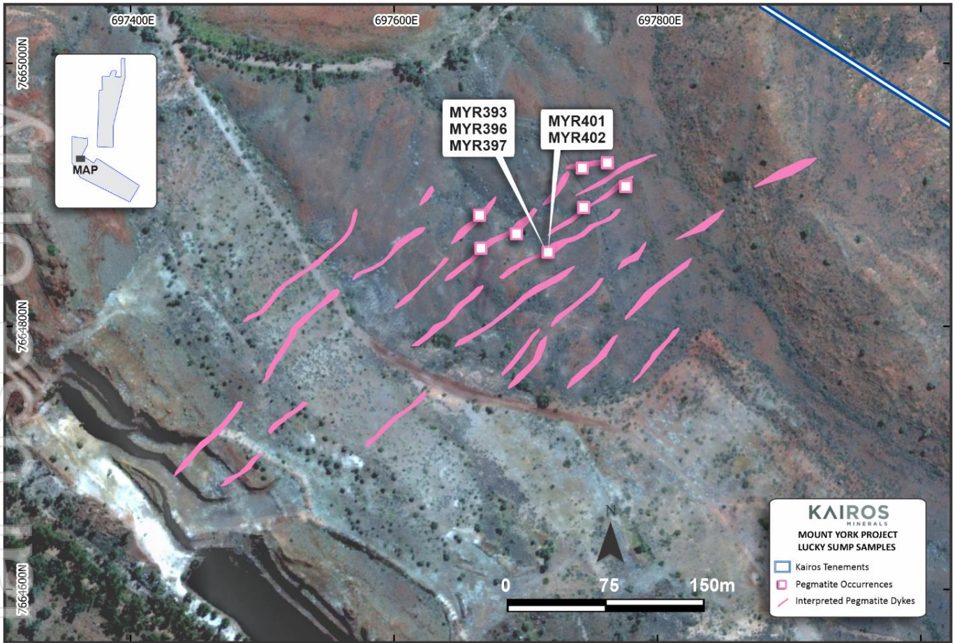
Figure 5. Detailed aerial image of the Lucky Sump Prospect showing the sample sites, mapped pegmatite occurrences within the interpreted pegmatite swarm. The interpreted dyke swarm is based on processed images of the RGB aerial scene. The dyke swarm is interpreted to be largely under shallow cover.
