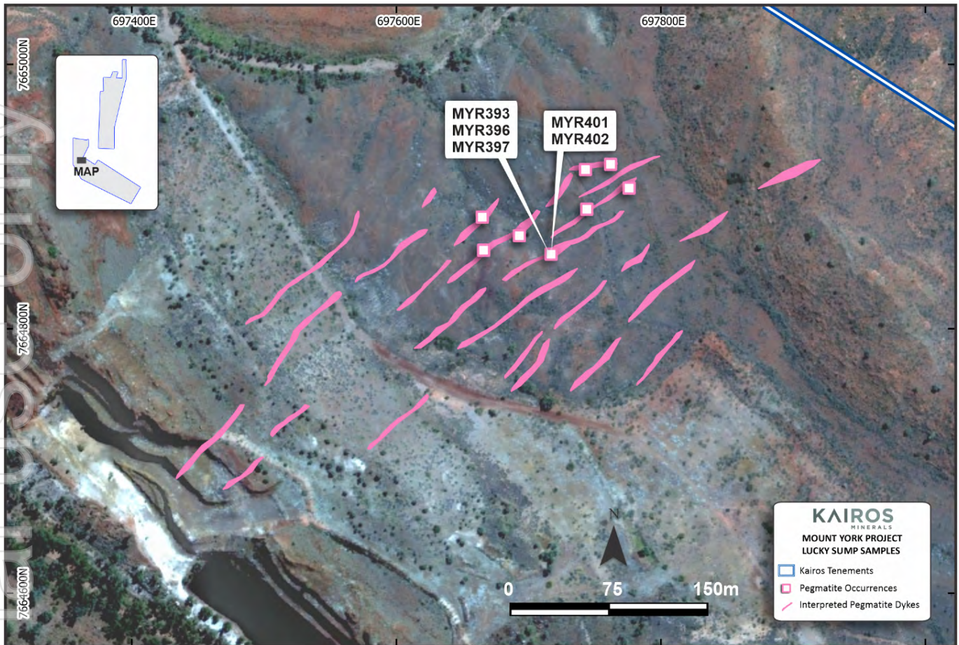
Figure 6. Detailed aerial image of the Lucky Sump Prospect showing the sample sites, mapped pegmatite occurrences within the interpreted pegmatite swarm. The interpreted dyke swarm is based on processed images of the RGB aerial scene. The dyke swarm is interpreted to be largely under shallow cover.
