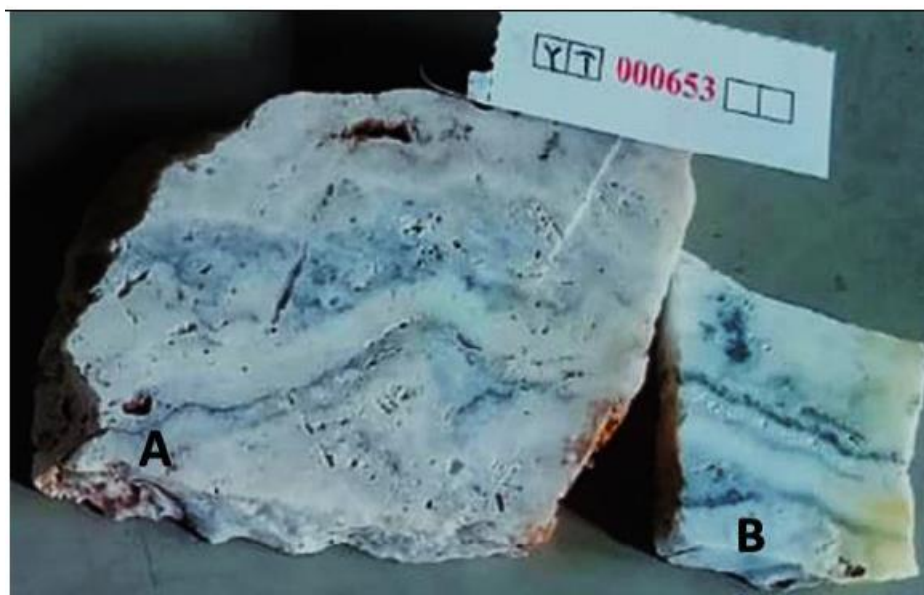
Figure 5: Sample of quartz vein from Aloe Eumpeuk prospect area. The samples show the occurrence of dark-grey, finely-laminated, sulphide-gold bearing ginguro bands
