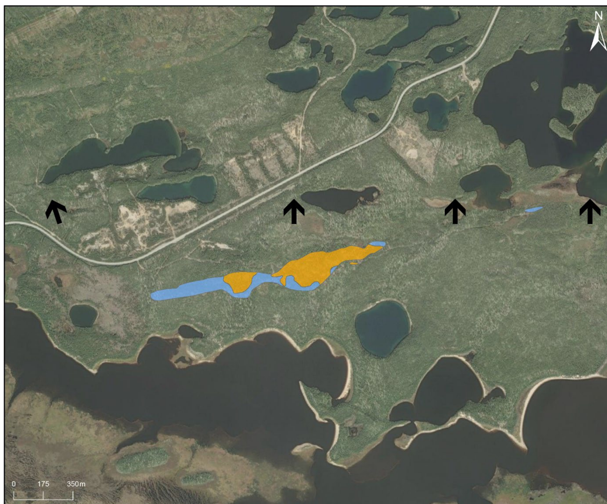
Figure 4 - Pegmatite delineation and mineralised zonation over 1,200m at Cancel with arrows showing where ore body remains open
