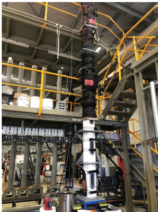
Image 16 / Nifty 6m high metallurgical test work column
