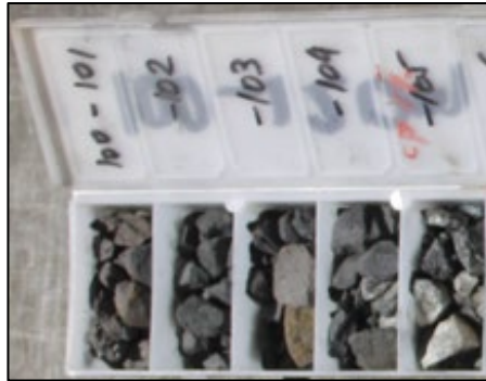
Image 18 / RC drill chips: 21MDRC027, 86-106m (20m @ 1.60 % Cu & 794 ppm Co, transitional to sulphide chalcopyrite and chalcocite mineralisation)
