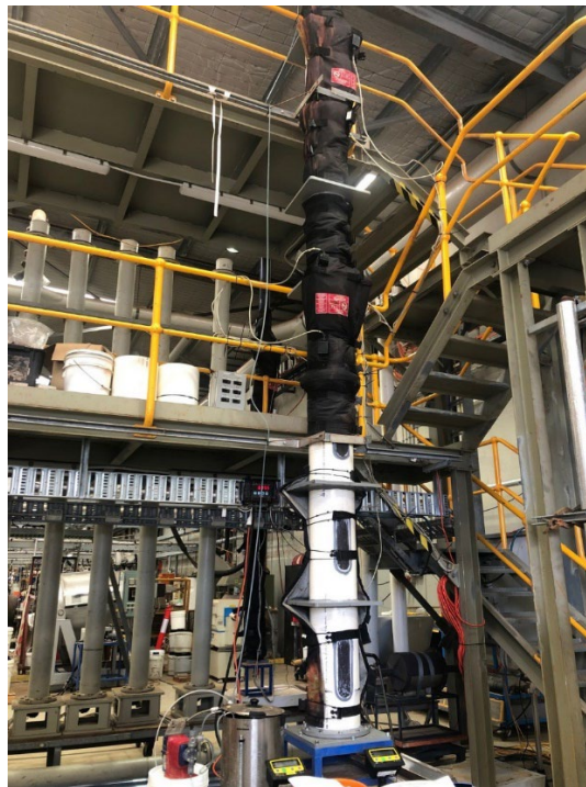
Image 16 | Nifty 6m high metallurgical test work column
