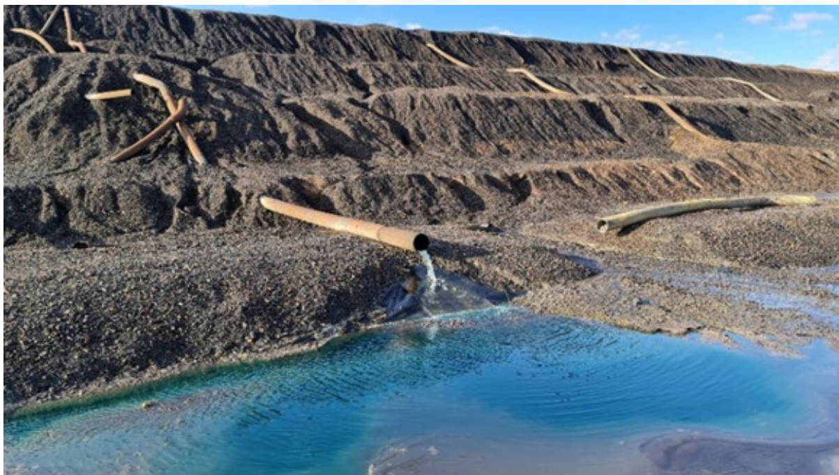
Image 14 / Copper rich solution flowing out of the heaps following recent rainfall at Nifty
