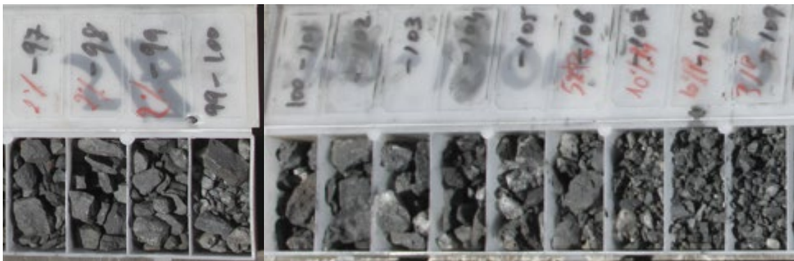
Image 17 / RC drill chips: 21MDRC030, 96-109m (13m @ 1.77 % Cu & 818 ppm transitional to sulphide chalcopyrite and chalcocite mineralisation)
