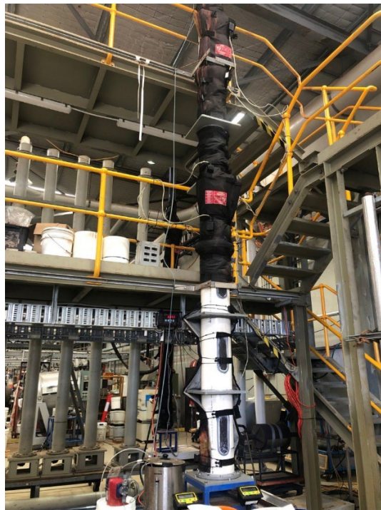
Image 16 | Nifty 6m high metallurgical test work column
