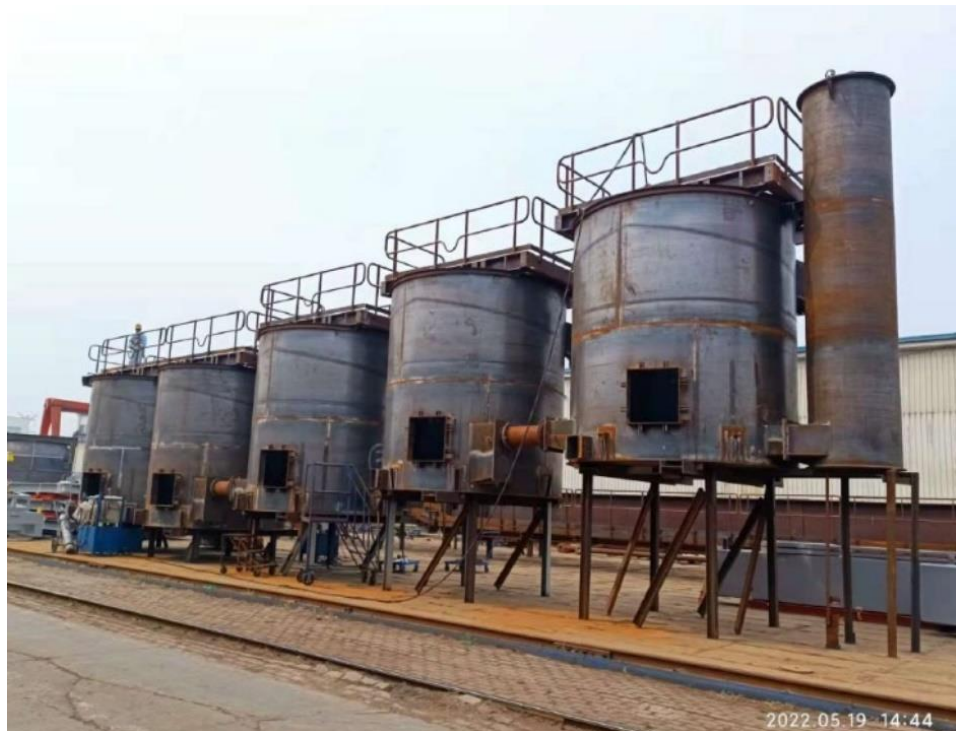
Figure 7. Flotation cell trial assembly in May prior to shipping.
