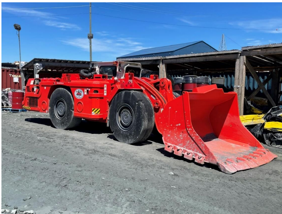
Figure 2: Commencement of fleet replacement with arrival of a Sandvik LH307 loader
