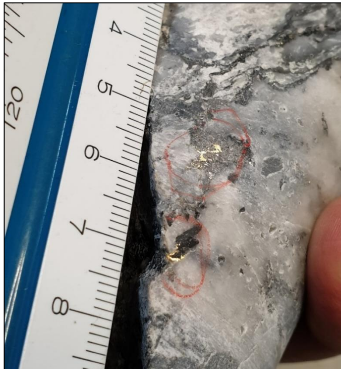
Figure 1: Visible gold within an interval that assayed 0.25 metres at 972g/t gold in diamond drill hole 22GZL9016 testing the Gap Zone at the Morning Star Gold Mine.
