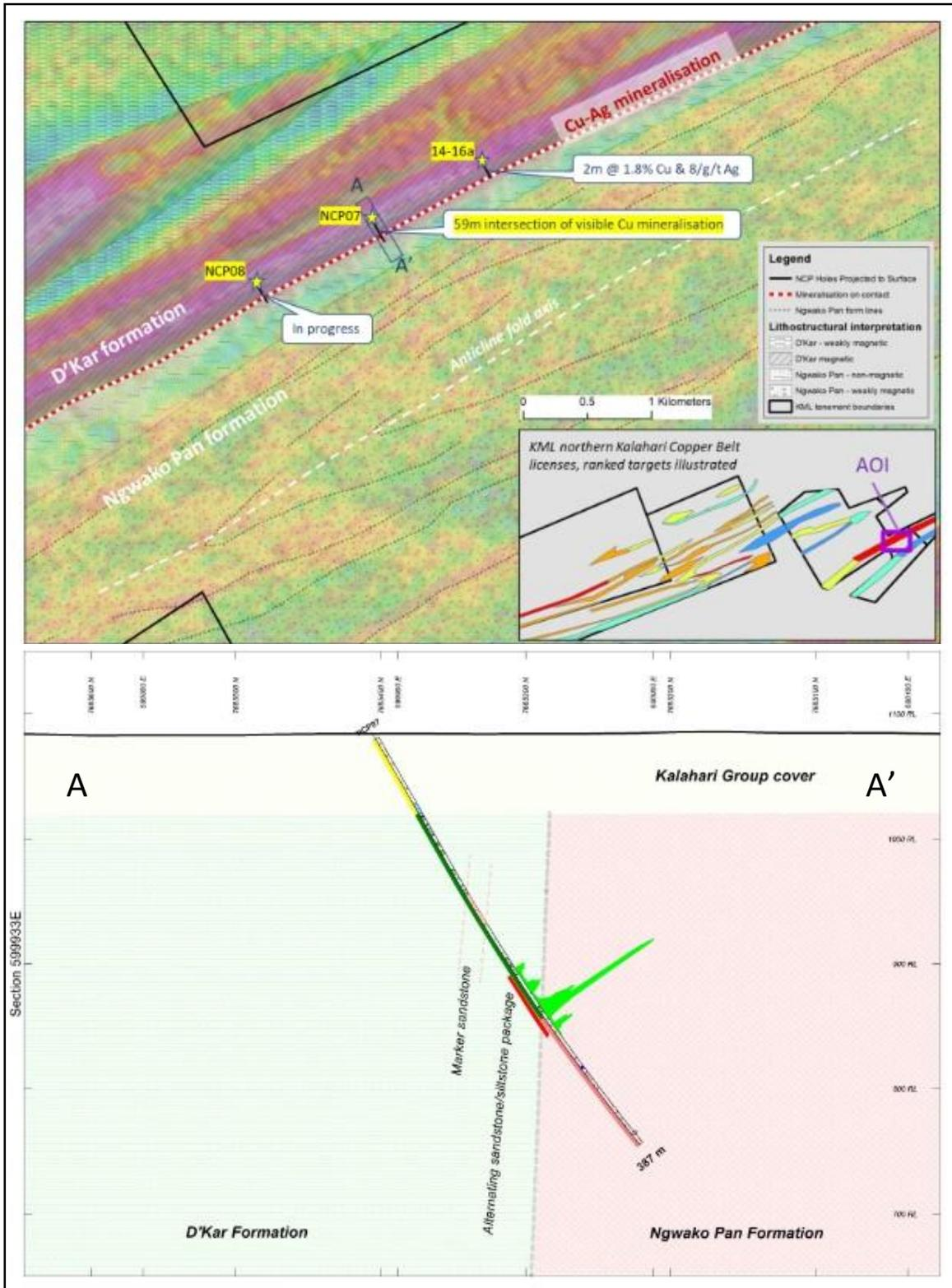
**Figure 4.** Plan view (above) illustrating drill positions on airborne magnetic data. Section (below) through NCP07 illustrating mineralisation (green plot) related to the D'Kar / Ngwako Pan formation contact.
