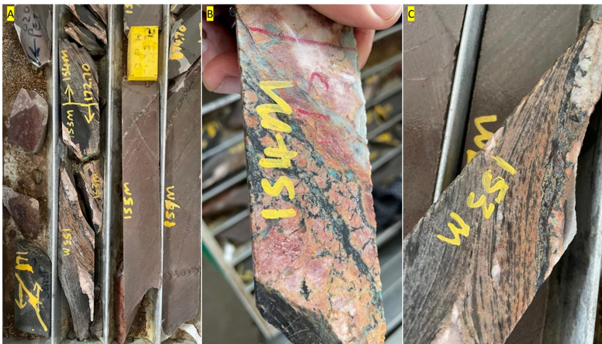
Figure 2. Examples of vein-hosted chalcocite mineralisation from historical hole TRDH14-16a (grey metallic mineral) which returned grades of 2m @ 1.8% Cu and 8 g/t Ag.
