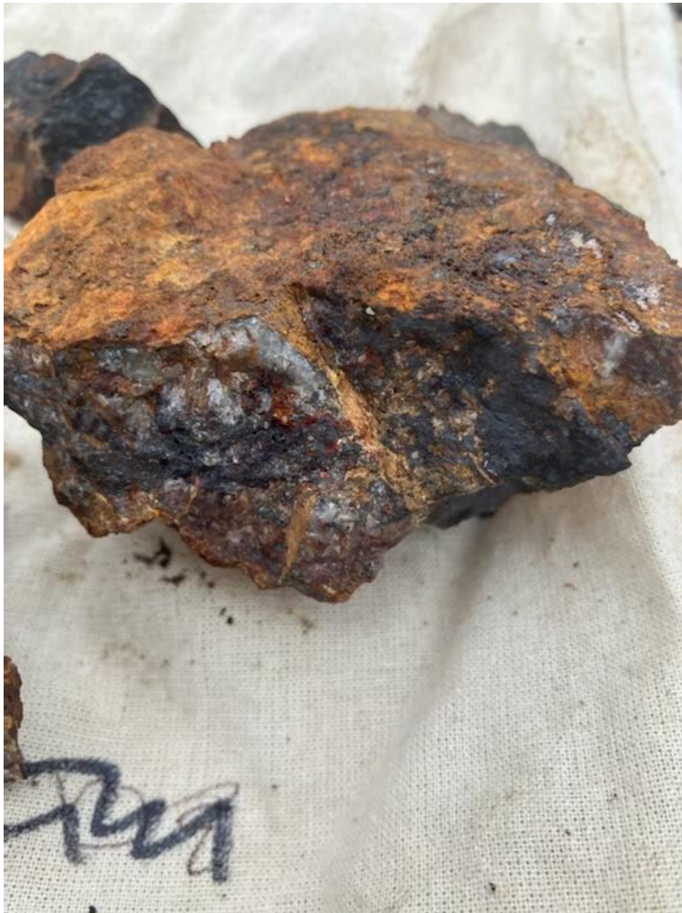
Figure 1 Rock Sample DPRC016 (Zone 1: Gossanous-brecciated crystalline prismatic quartz veining)
