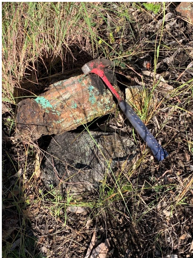
Figure 3 Zone 1 mineralisation – layered vuggy quartz, iron oxide and malachite gossan
