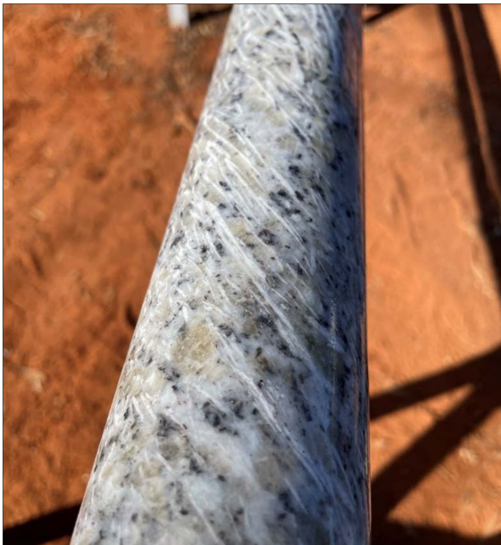
Figure 5. Image of the Manna Lithium Projects Lithium bearing Pegmatite showing spodumene crystals throughout the core. Hole MRCD0038 at a depth of 169m
