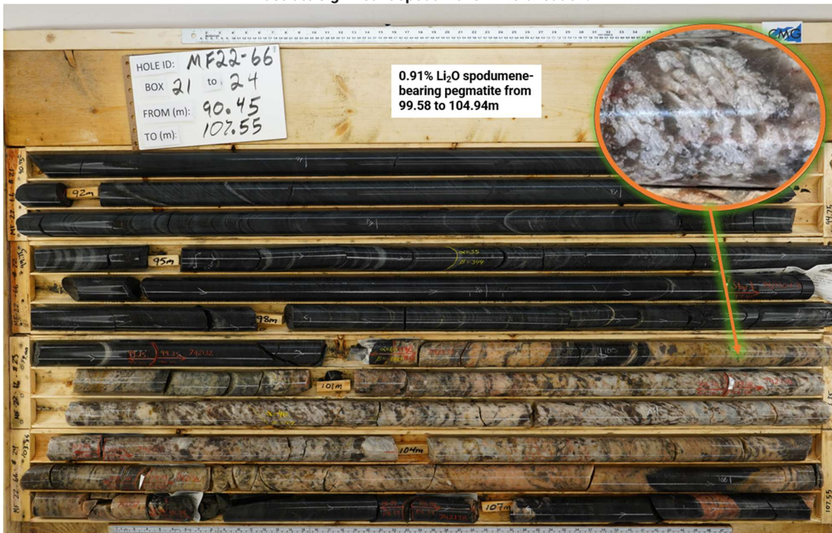
Figure 6: White pegmatite hosts spodumene laths intersected from 99.58 to 104.94m depth in Hole MF22-66. Close-ups illustrate significant spodumene mineralisation.
