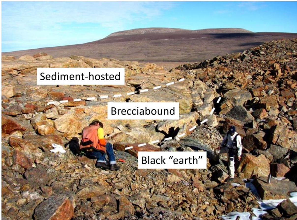
Figure 5: Mineralisation types of the Discovery Zone Note: The photo is of the 2010 field campaign.
