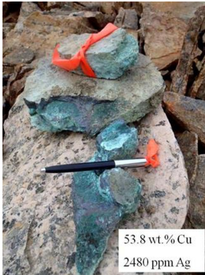
Figure 6: Breccia bound copper mineralisation
