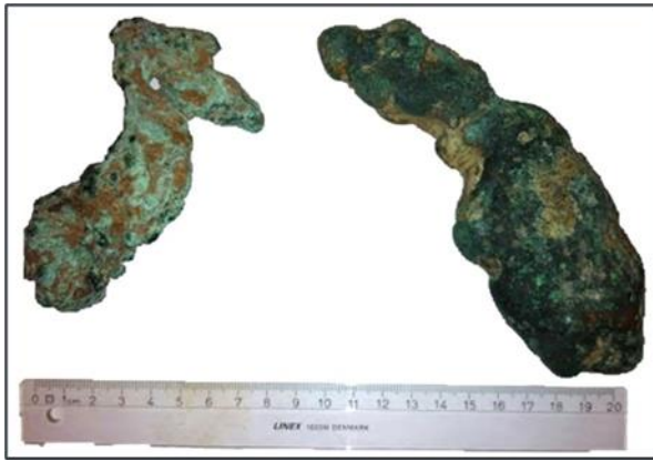
Figure 10: Large native copper specimens from ARC. Sample on the right weighs ~1 kg
