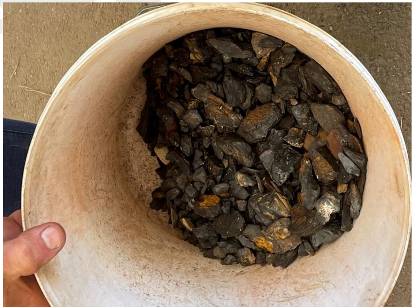
Figure 16: Manganese ore concentrate
