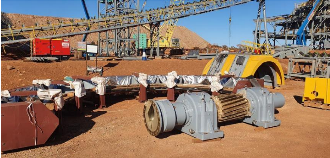
Figure 9 – Ball mill gear & pinion.
