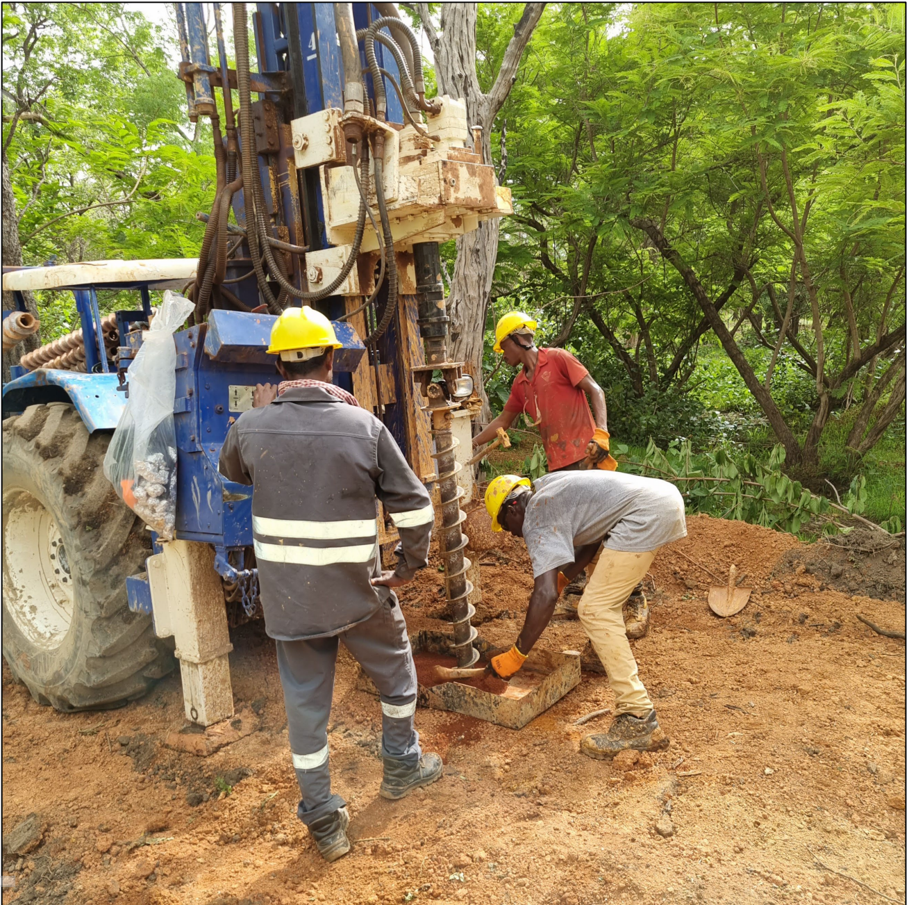
Figure 4: Infill auger drilling on the Kada Gold Project at Bereko Prospect, 7km north of the ~930,000oz Mineral Resource area at Massan Prospect.
