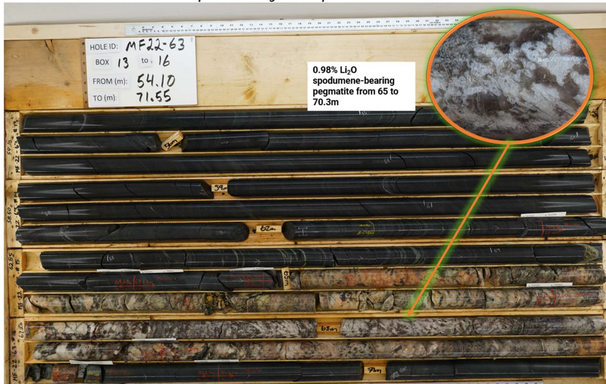
Figure 3: White pegmatite hosts spodumene laths intersected from 65 to 70.3m depth in Hole MF22-63 (Hole 04). Close-ups illustrate significant spodumene mineralisation.
