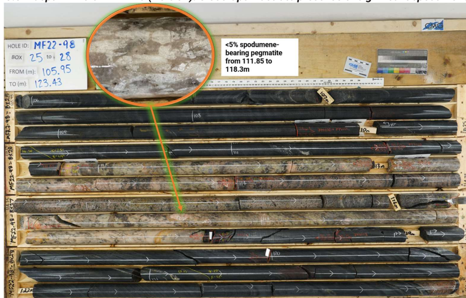
Figure 7: White pegmatite hosts approximately <5% of fine to large, white-grey, spodumene laths intersected from 111.85 to 118.3m depth in Hole MF22-98 (Hole 39). Close-ups illustrate presence of significant spodumene
