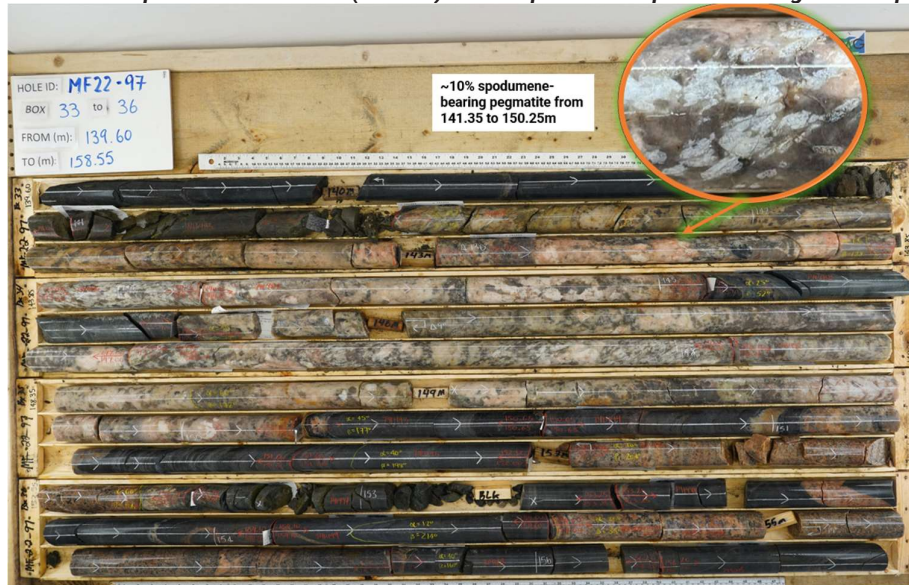
Figure 6: White pegmatite hosts approximately 10% of fine to large, white-grey, spodumene laths intersected from 141.35 to 150.25m depth in Hole MF22-97 (Hole 38). Close-ups illustrate presence of significant spodumene
