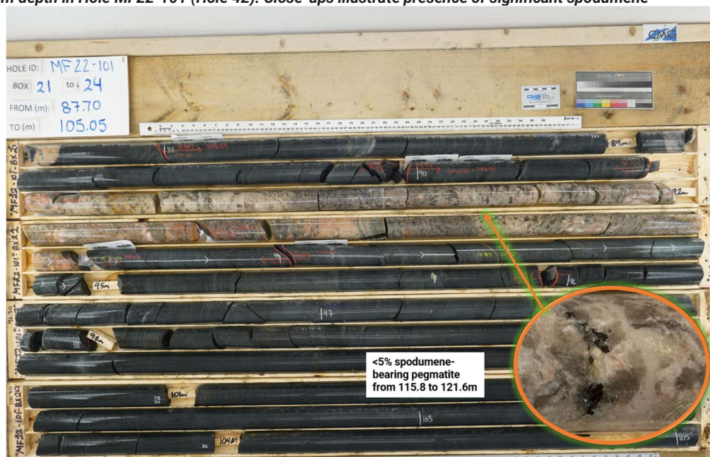
Figure 9: White pegmatite hosts approximately <5% of fine to large, white-grey, spodumene laths intersected from 115.8 to 121.6m depth in Hole MF22-101 (Hole 42). Close-ups illustrate presence of significant spodumene
