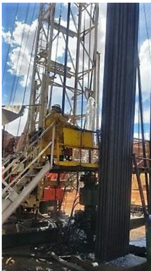
Figure 1: Supersaturated brine free flowing direct from the Cane Creek 32-1 well up the tubing.
