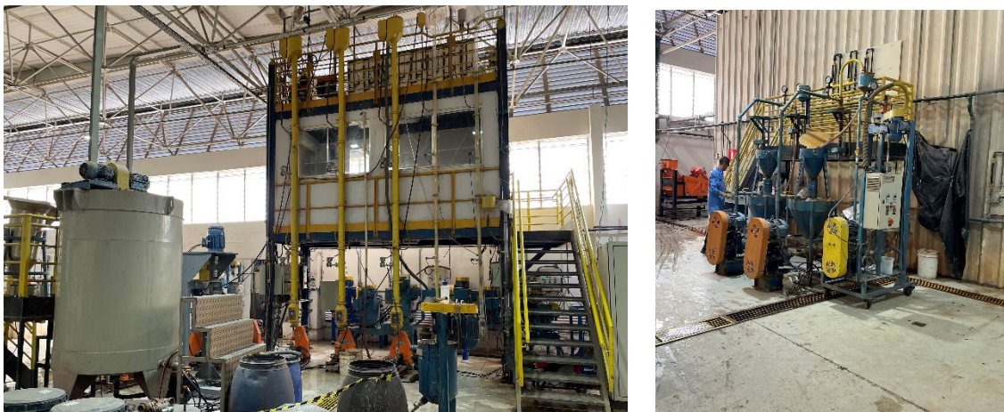
Figure 4: Metallurgical laboratory showing DMS and flotation columns and other equipment, Belo Horizonte, Brazil
