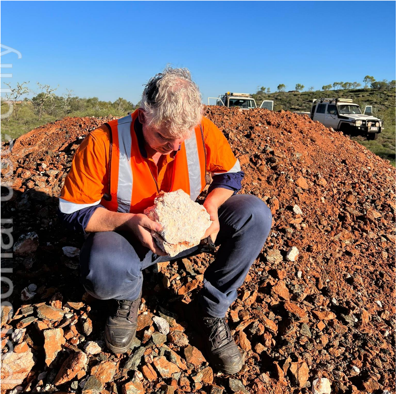
Figure 2. with Kairos Managing Director and Geologist Peter Turner examining pegmatite samples from recent earthmoving activities at the Lucky Sump Prospect. Host rocks to the pegmatites appear to be basaltic-gabbroic rocks. The pegmatite samples have been excavated from their source below the sump and are not considered transported.
