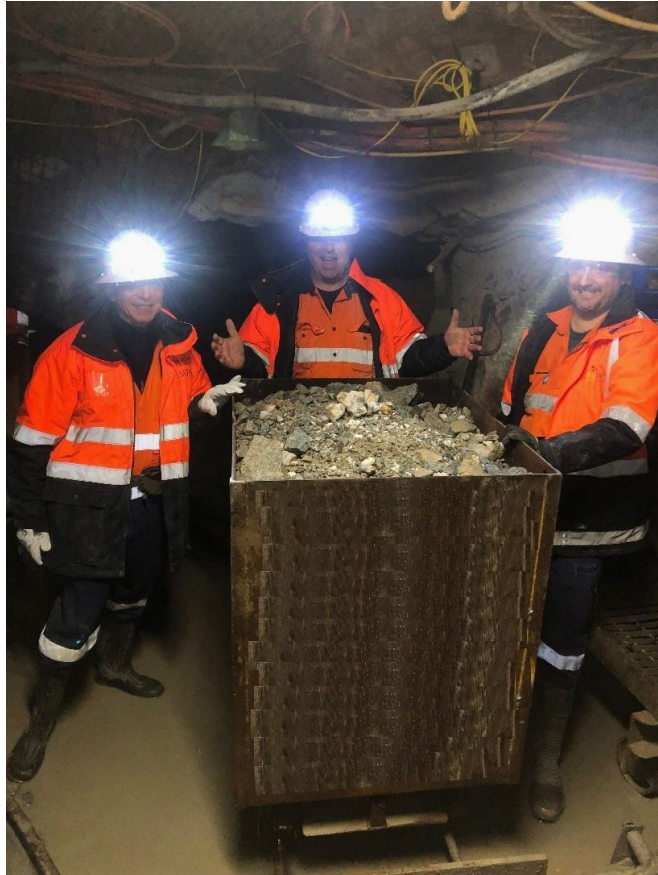
Figure 10: An ore “truck” on the main haulage 9 Level ready to be hoisted to the surface
