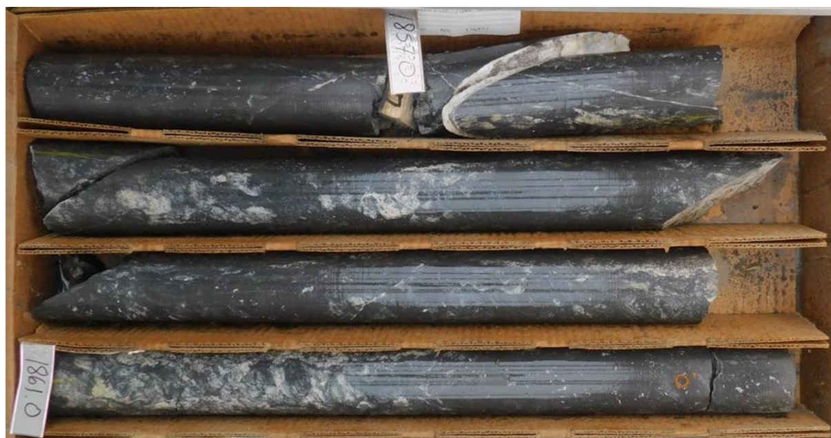
Figure 3: Photo of massive sphalerite (zinc sulphide – black/brown) and magnetite (black) in drill hole WD22-05 at approximately 566 – 567.2m (1857 – 1861ft) downhole.
