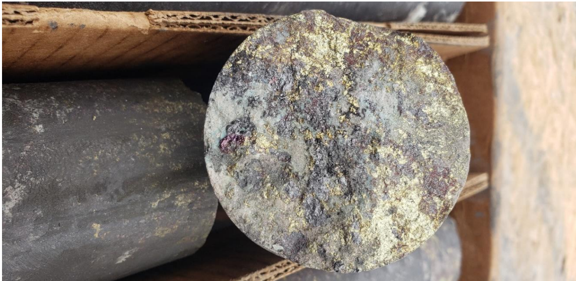
Figure 1: Photo of chalcopyrite and bornite (copper sulphide) within magnetite skarn In from approximately 363.91m (1194ft) downhole in drill hole WD22-05.
