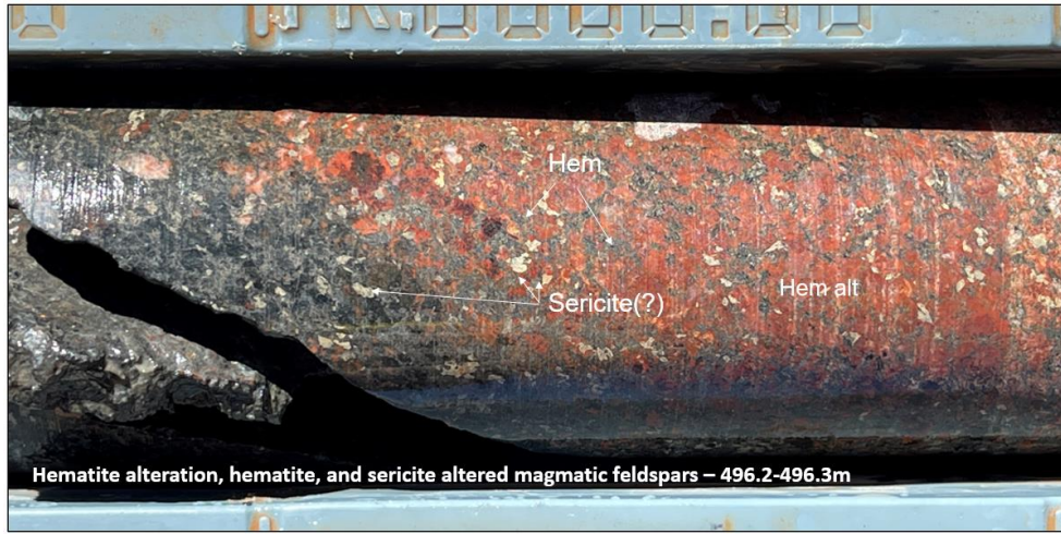
Figure 3: Hematite alteration of the igneous host rock. Similar to the alteration found around other IOCG deposits in Australia
