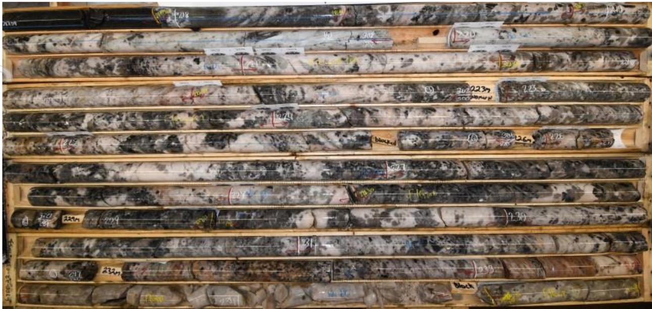
Figure 2: Diamond core from Phase 2 North Aubry (Seymour) drill hole GTDD-22-0323 (217.6 – 236.6m downhole depth)
