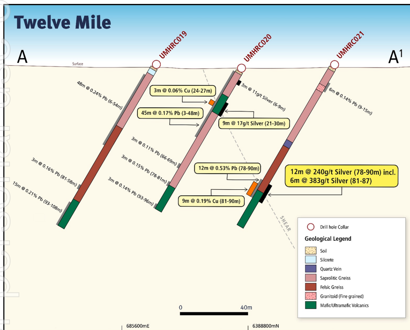
Figure 4: Section through Twelve Mile prospect showing significant intersections of silver, copper and lead. Note: Zinc intersections not included for clarity. Refer to Appendix 2 for table of results.
