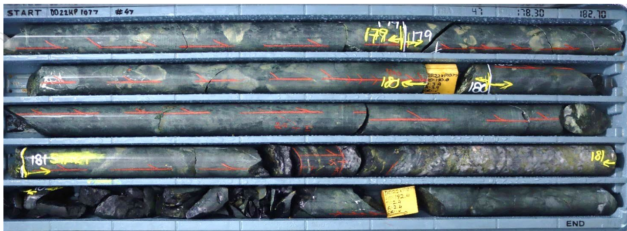
Figure 3: DD22KP1077 intersected 5m @ 3.43 g/t Au, 0.47 % Cu, 5.16 g/t Ag from 181m with massive sulphide (pyrite 40% and chalcopyrite 40%) and quartz veining between 181.4m – 182m. Mineralisation is hosted within Annabelle Volcanics and in this instance is situated at the contact between an andesitic agglomerate (large, coarser rock fragments) and finer grained pyroclastic units.
