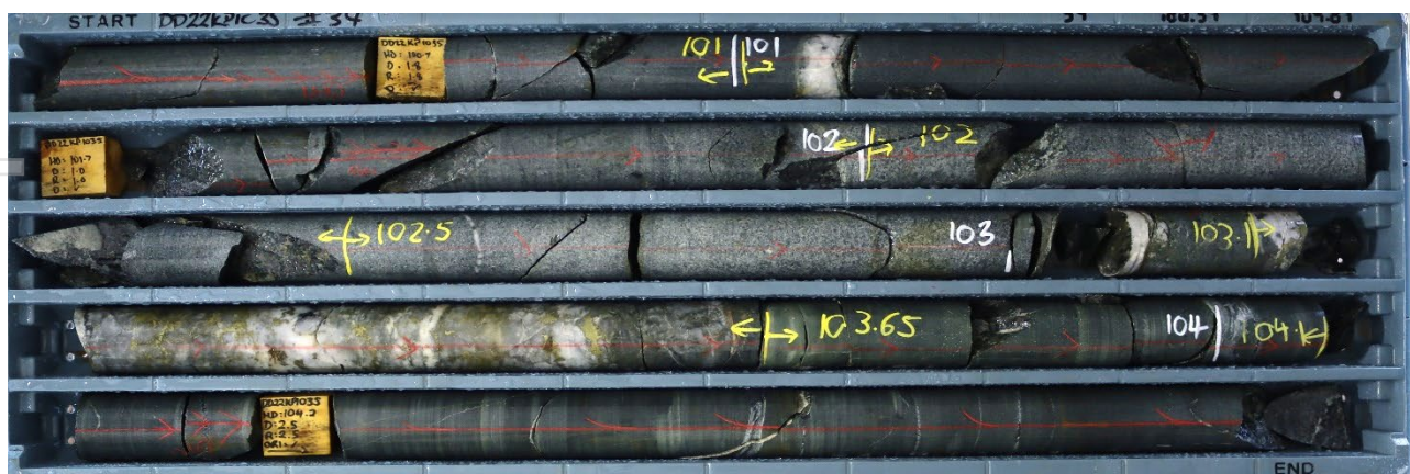
Figure 4: DD22KP1035 intersected 0.55m of quartz-sulphide (20% pyrite, 15% chalcopyrite) veining between 103.1m-103.65m that returned 62.6 g/t Au, 4.27 % Cu, 48.4 g/t Ag. Stringer sulphides and chlorite alteration were observed in the footwall to the vein. Mineralisation is situated at the contact between tonalite in the hangingwall and an andesitic porphyry intrusive unit.
