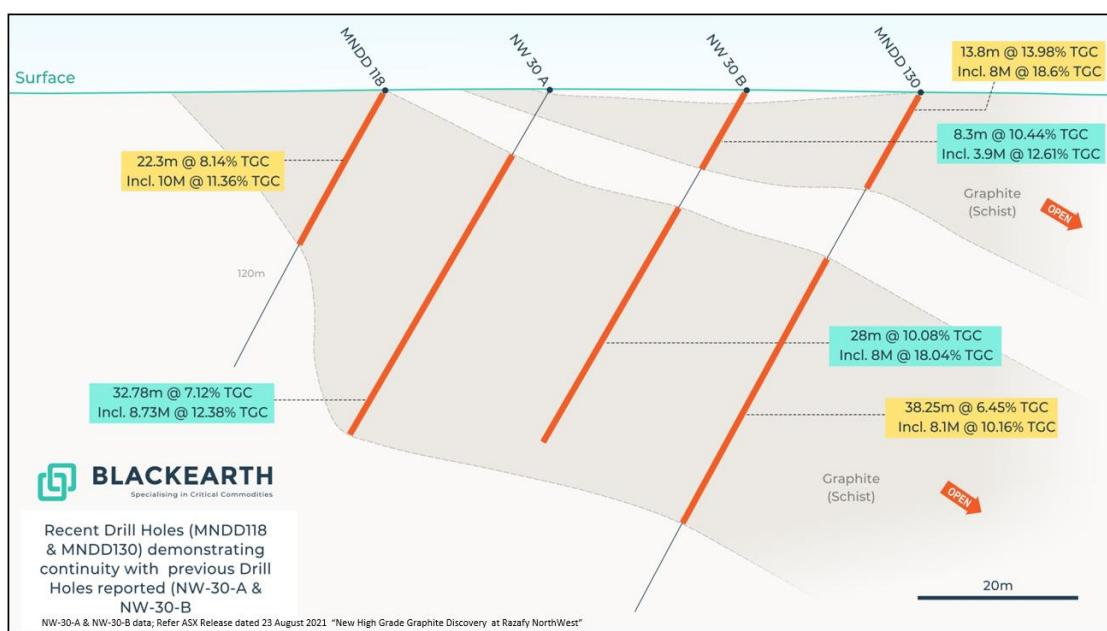
Figure 1: Razafy North West - Drilling Cross-section (A-B)
