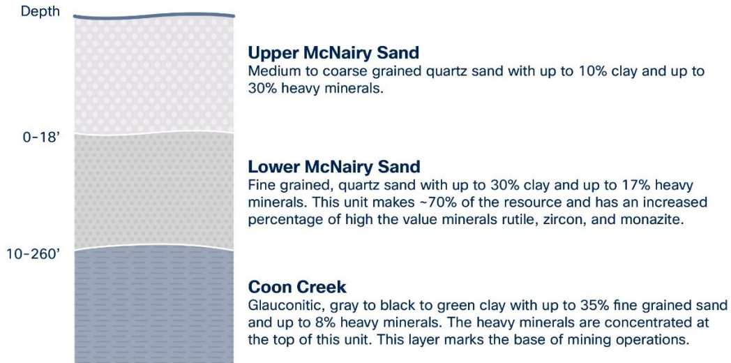
Figure 21: Idealized cross-section of McNairy Sand.
