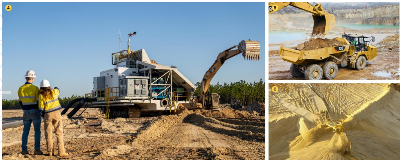
Figure 23: A – Example mobile mining unit mineralized material feed (courtesy of Mineral Technologies); B – Example dry mining of waste; C – Example wet sand tails waste.
