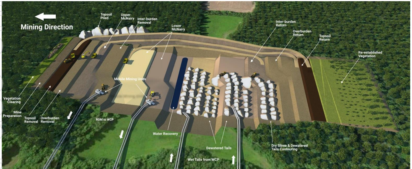
Figure 22: Titan Project mining cycle.
