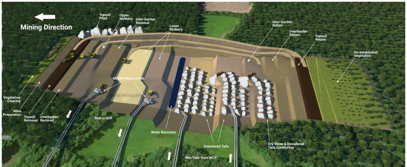
Figure 13: Titan Project mining cycle.
