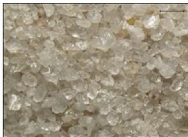
Figure 2: Micrographs indicated clean product after final magnetic separation testwork.
