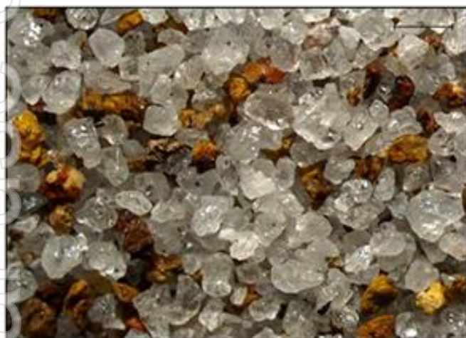
Figure 2: Micrographs indicated clean product after final magnetic separation testwork.
