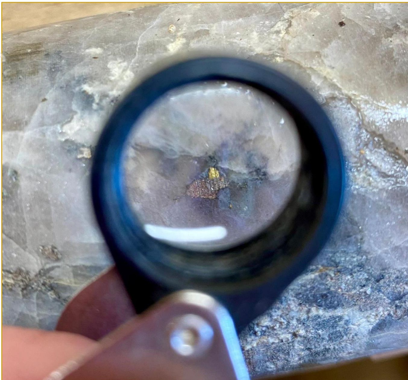
Figure 12. RPM-008 115.8m – Visible Gold in a quartz-sulfide vein within intrusive rocks.
