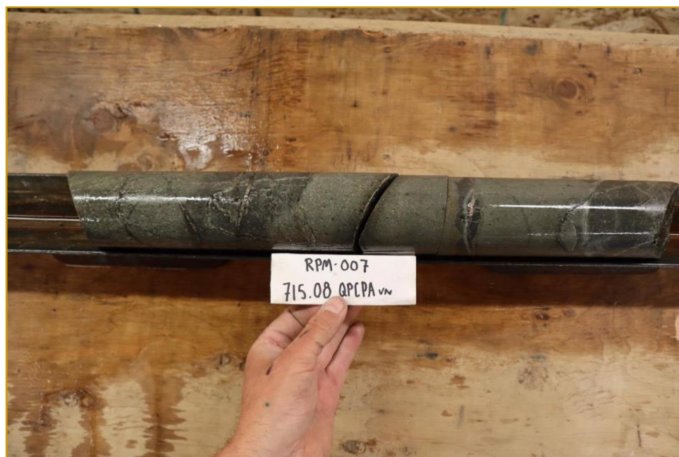
Figure 5. RPM-007 218m – Strongly mineralized quartz-sulfide veins containing arsenopyrite within hornfels unit. Strong dark hydrothermal tourmaline alteration halo around mineralized veins. (Note: depth written on boxes in feet)
