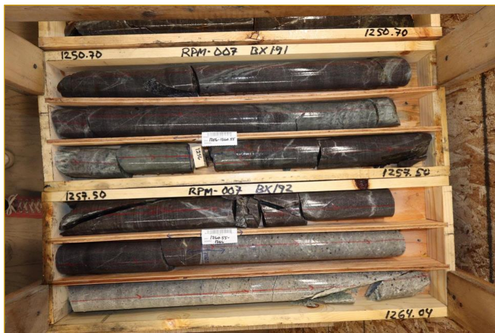
Figure 4. RPM-007 381.3 - 385.4m – moderately mineralized sheeted veins and shears near the Hornfels-Intrusive contact. (Note: depth on boxes in feet)
