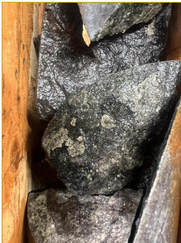
Figure 6. RPM-007 135.1m Strongly mineralized hornfels with chunky arsenopyrite
