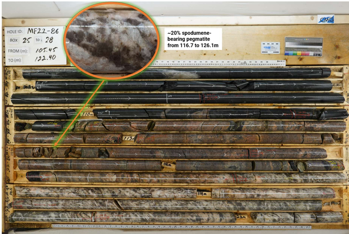
Figure 3: White pegmatite hosts approximately 20% of fine to large, white-grey, spodumene crystals intersected from 116.7 to 126.1m depth in Hole MF22-86 (Hole 27). Close-ups illustrate presence of significant spodumene
