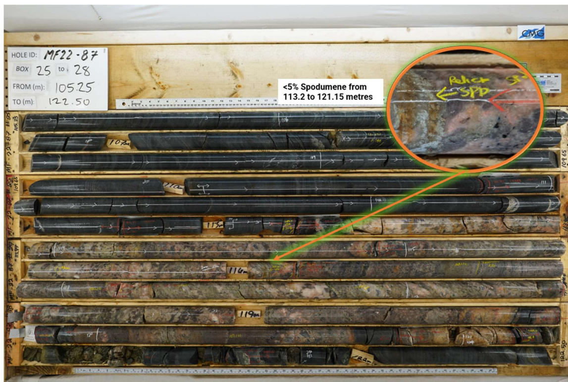
Figure 4: White pegmatite hosts approximately <5% of fine to large, white-grey, spodumene crystals intersected from 113.2 to 121.15m depth in Hole MF22-87 (Hole 28). Close-ups illustrate presence of significant spodumene
