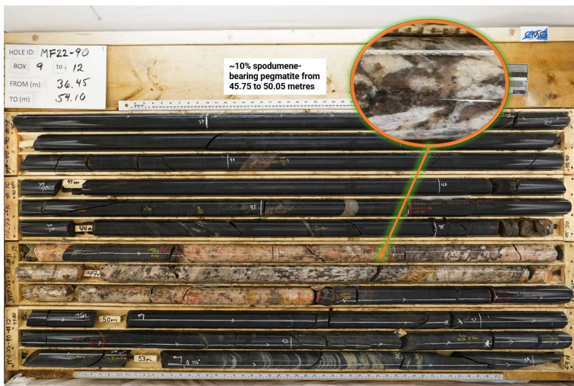
Figure 7: Two white pegmatites hosts approximately ~10% of fine to large, white-grey, spodumene crystals intersected from 45.75 to 49.05m depth in Hole MF22-90 (Hole 31). Close-ups illustrate significant spodumene
