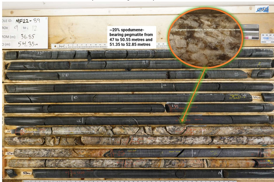
Figure 6: Two white pegmatites hosts approximately ~20% of fine to large, white-grey, spodumene crystals intersected from 47 to 50.55 and 51.35 to 52.85m depth in Hole MF22-89 (Hole 30). Close-ups illustrate presence of significant spodumene
