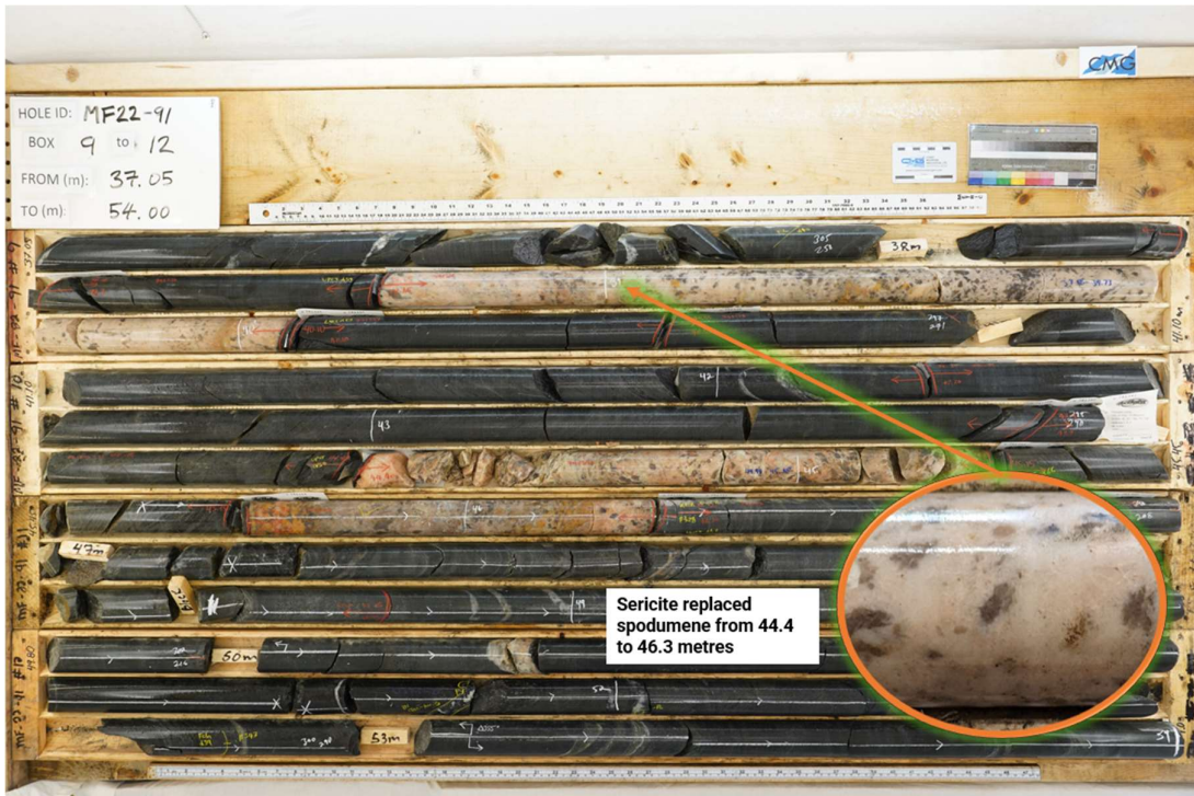
Figure 8: White pegmatite hosts sericite mineralisation replacing spodumene from 44.4 to 46.3m depth in Hole MF22-91 (Hole 32). Close-ups illustrate barren pegmatite
