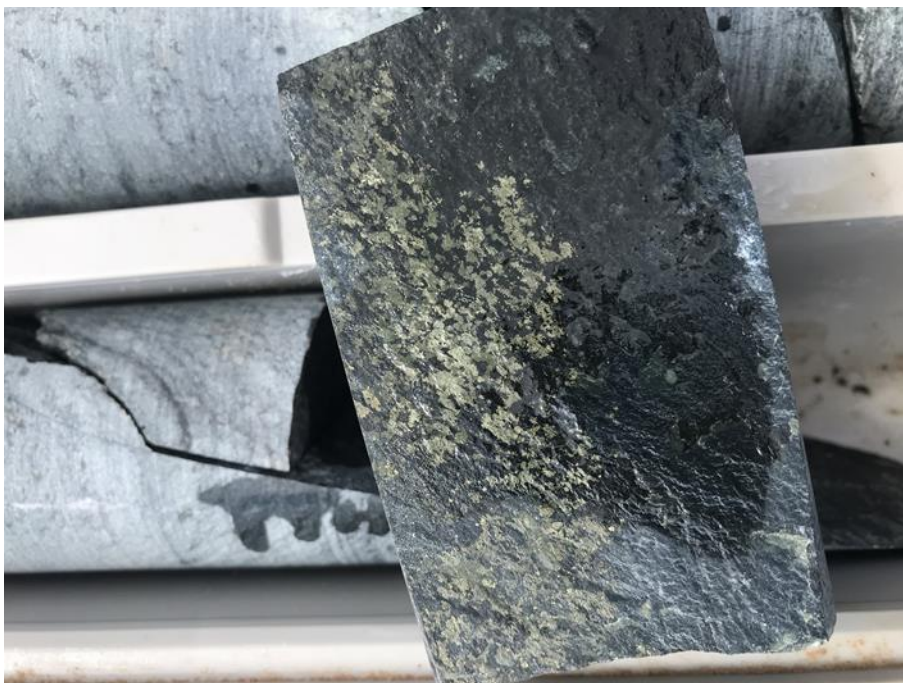
Figure 10 - Diamond Hole - NRDD004 - Nickel and Copper in sulphide at 508.0m
