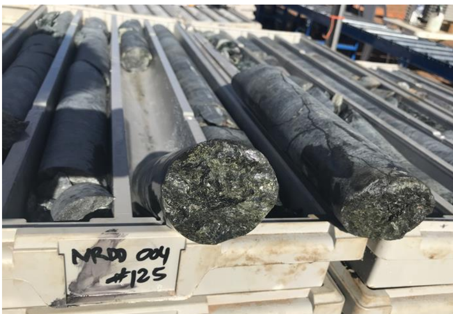
Figure 8 - Diamond Hole - NRDD004 – Nickel and Copper mineralisation 436.85 – 440.3m
