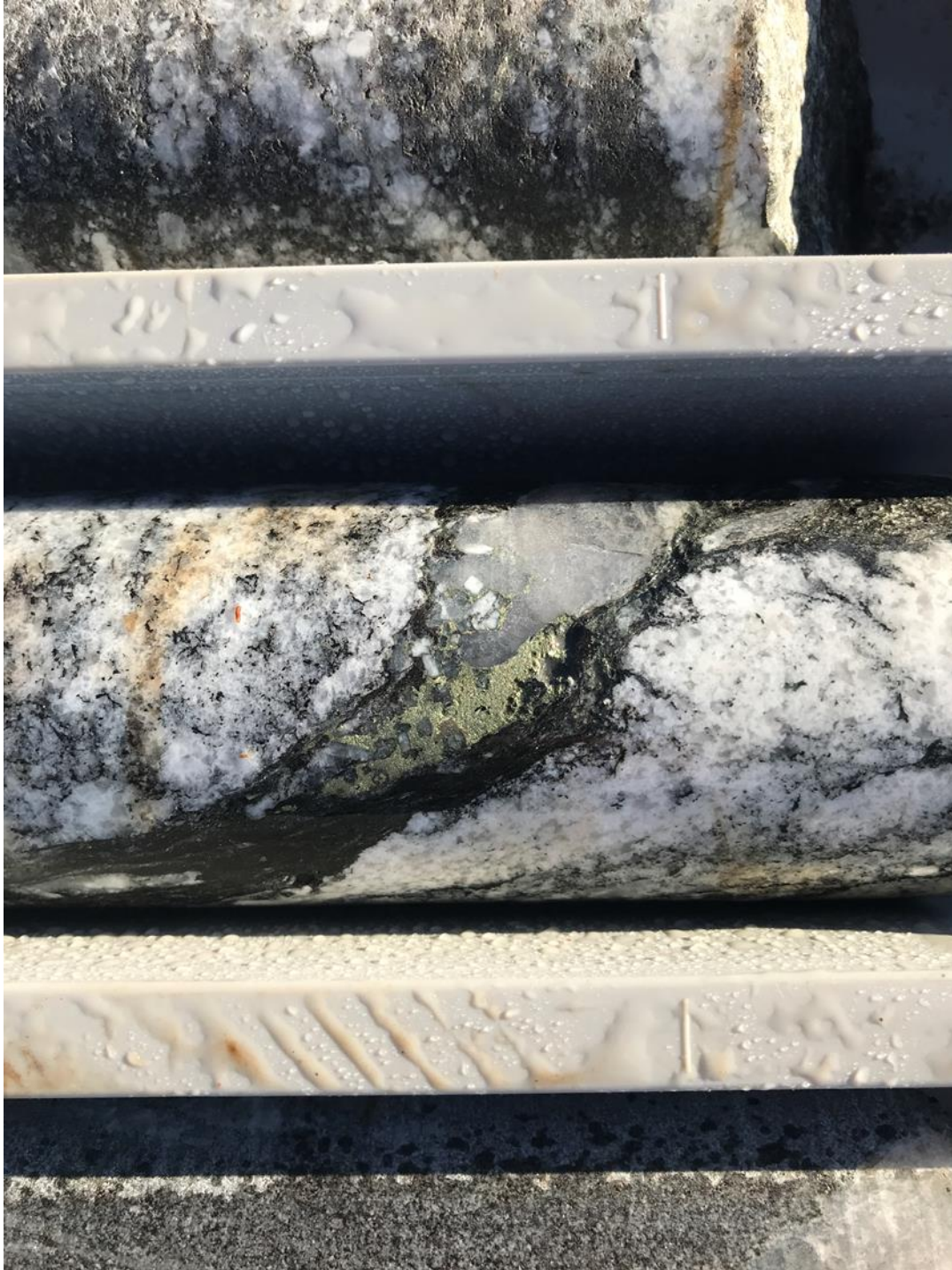
Figure 6 – Diamond Hole -NRDD004 – Copper, Silver and Zinc mineralisation in sulphide at 342.9m
