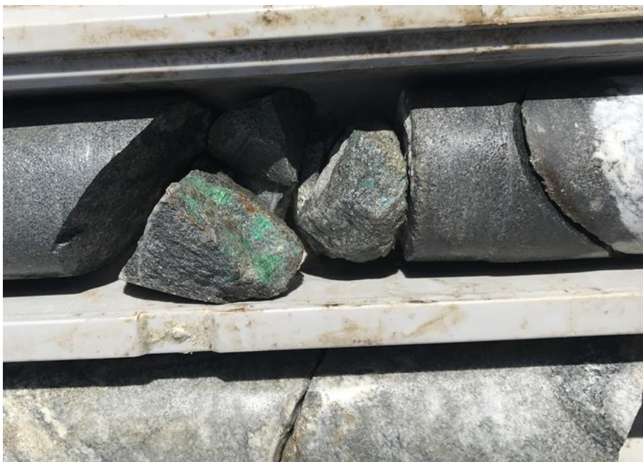
Figure 7 – Diamond Hole - NRDD004 - Copper, Silver and Zinc mineralisation at 367.4m
