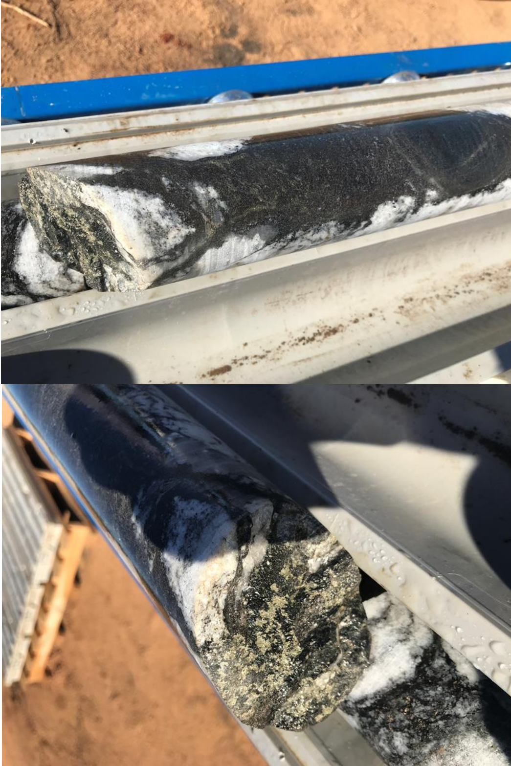
Figure 5 – Copper, Silver and Zinc mineralisation in sulphide at 340.75m
