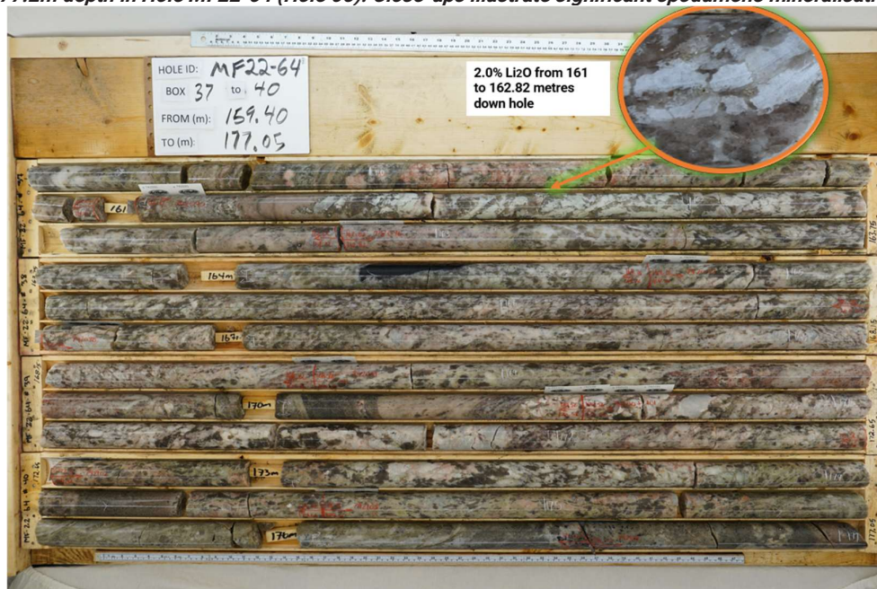
Figure 1: White pegmatite hosts fine to medium, white-grey, spodumene crystals intersected from 159.1 to 177.2m depth in Hole MF22-64 (Hole 05). Close-ups illustrate significant spodumene mineralisation.
