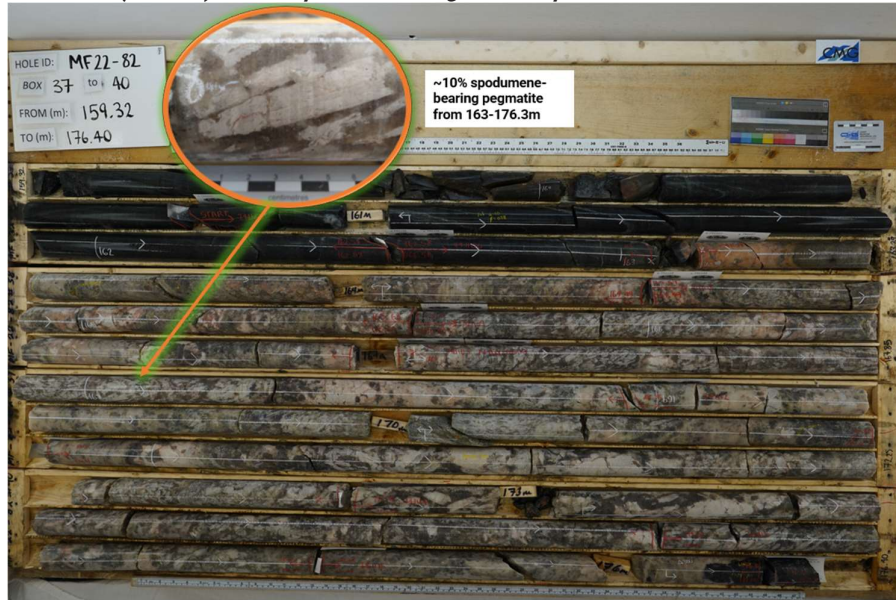
Figure 4: White pegmatite hosts fine to medium, white-grey, spodumene crystals intersected from 163 to 176.2m depth in Hole MF22-82 (Hole 23). Close-ups illustrate significant spodumene intervals
