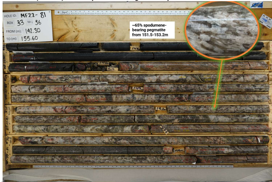
Figure 3: White pegmatite hosts fine to medium, white-grey, spodumene crystals intersected from 146 to 160.7m depth in Hole MF22-81 (Hole 22). Close-ups illustrate significant spodumene intervals
