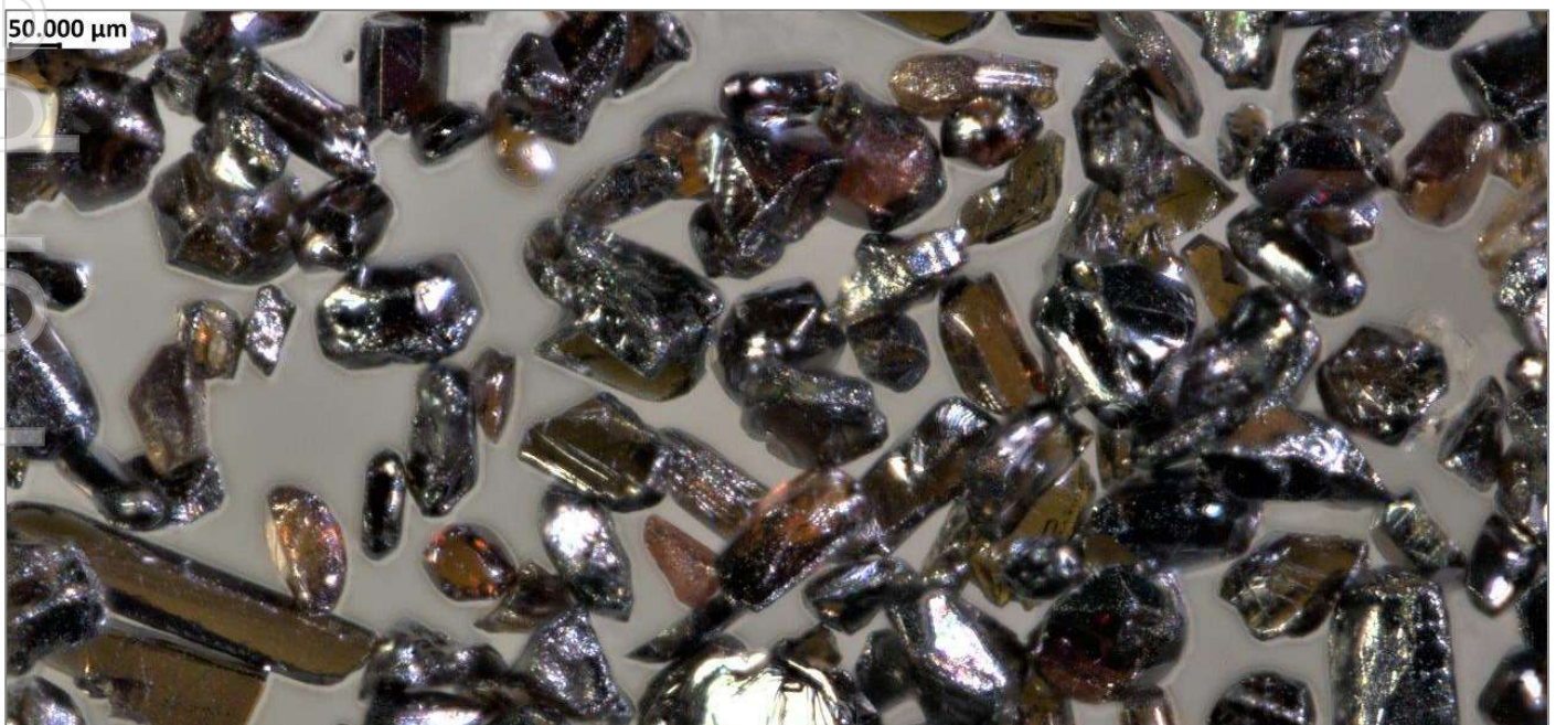
Figure 26: Photomicrograph of high purity rutile product
