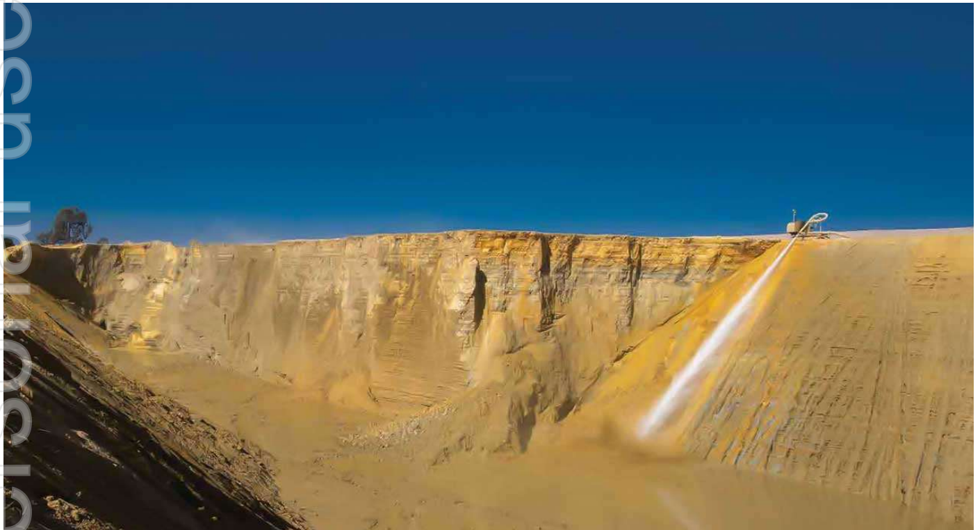
Figure 20: Top-down hydro mining in operation (Source: Fraser Alexander)
