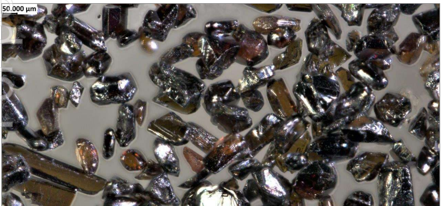
Figure 26: Photomicrograph of high purity rutile product
