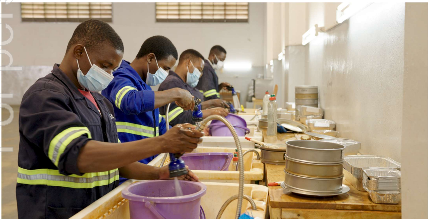
Figure 50: Sample de-sliming at the Company's laboratory facility in Malawi
