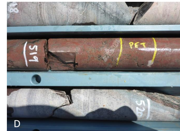
Above: BKDD001 selected drill core: A) top of basement contact (204m): B) fine grained, hematite bearing metasediment with quartz veining (242m): C) localised (3m downhole width) hematite – quartz – chlorite pervasive alteration – breccia texture (458m): D) zones of intense hematite veinlets (519m)
