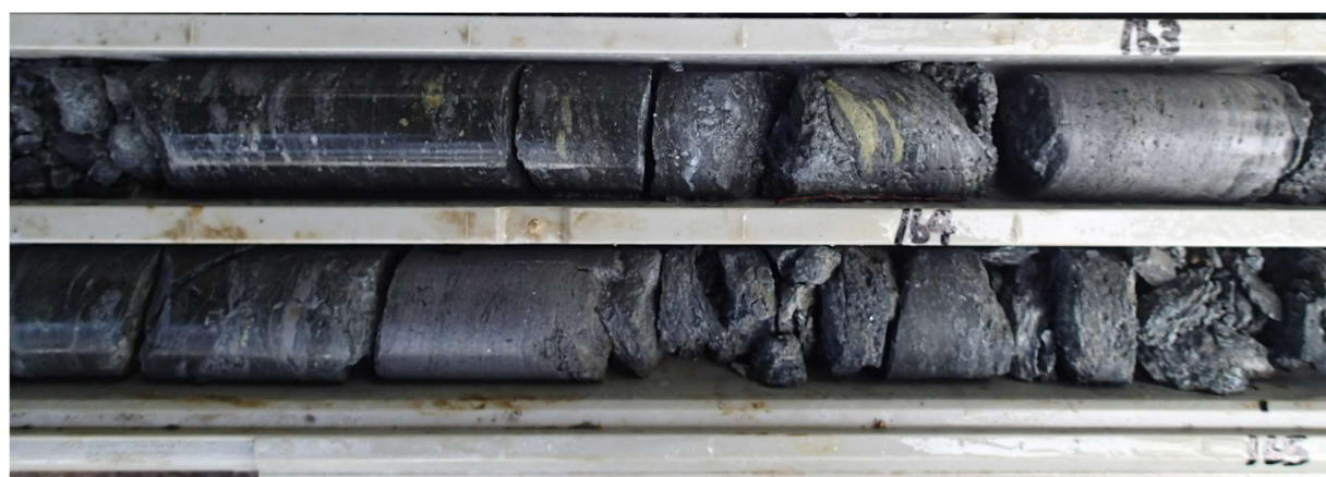
Figure 4: CRR21DD_016, detail from above Figure 3 of Samples (42)855 (top row) and (42)856 (bottom row) that extended from 163.20-165.10m downhole) exhibiting massive sulphide – sampled interval assayed 12.72% Zn, 6.25% Pb, 1.72% Cu, 44.62g/t Ag, 0.46g/t Au (NQ core, 50mm diameter)
