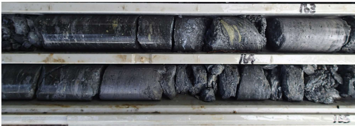
Figure 4: CRR21DD_016, detail from above Figure 3 of Samples (42)855 (top row) and (42)856 (bottom row) that extended from 163.20-165.10m downhole) exhibiting massive sulphide – sampled interval assayed 12.72% Zn, 6.25% Pb, 1.72% Cu, 44.62g/t Ag, 0.46g/t Au (NQ core, 50mm diameter)
