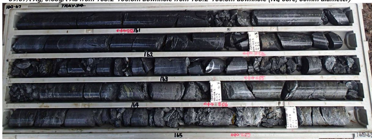
Figure 4: CRR21DD_016, detail from above Figure 3 of Samples (42)855 (top row) and (42)856 (bottom row) that extended from 163.20-165.10m downhole) exhibiting massive sulphide – sampled interval assayed 12.72% Zn, 6.25% Pb, 1.72% Cu, 44.62g/t Ag, 0.46g/t Au (NQ core, 50mm diameter)
